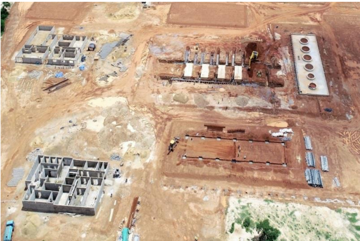
Photo 6: power station, HFO storage area.
