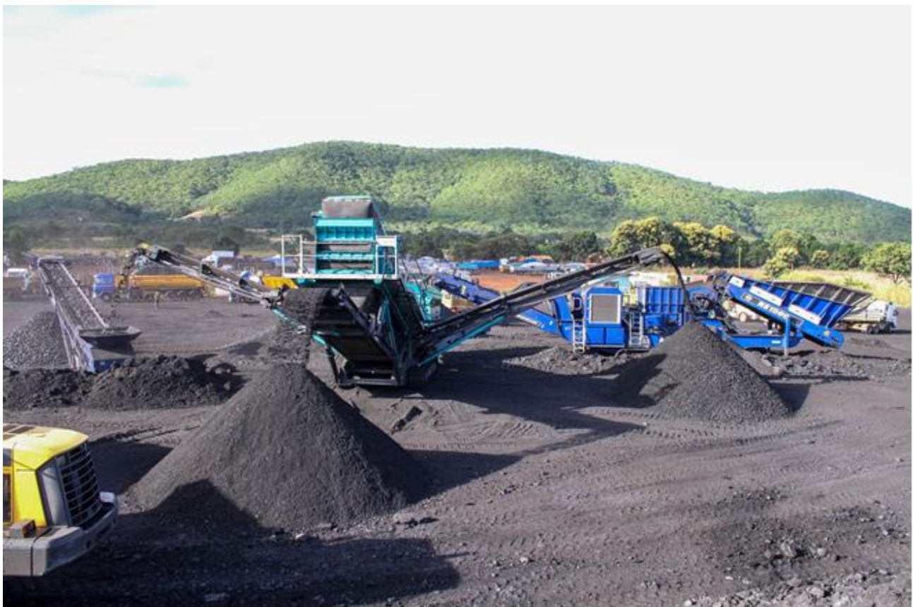
The stockpile area with coal being sized for different customers
