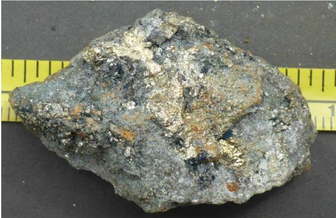
**Photo 10: Copper mineralisation, chalcocite ( $\text{Cu}_2\text{S}$ , black) associate with quartz-pyrite (outcrop sample)**
