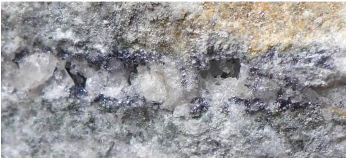
**Photo 9: Open textured (9mm wide) quartz-molybdenite (MoS<sub>2</sub>, molybdenum sulphide) vein (outcrop sample)**
