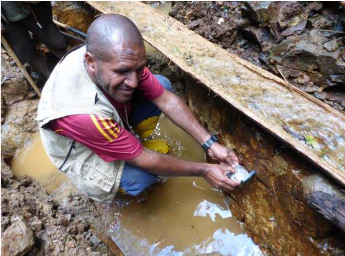
**Photo 15: Outcrop exposed beneath alluvial gold workings. Artisanal miners have started to mine hard rock mineralisation and recover gold by crushing and panning oxidised mineralisation in narrow, orthogonal veins sets (Gapsy measuring vein structures).**
