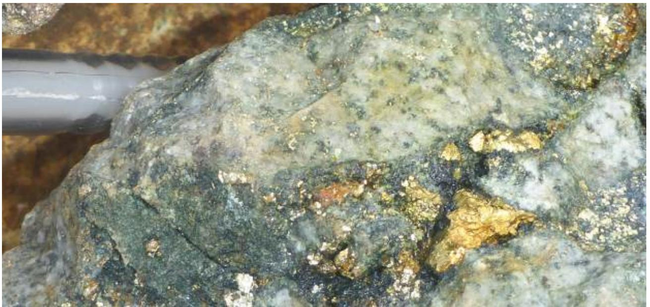
**Photo 11: The large system contains widespread phyllic (quartz-sericite-pyrite) alteration (outcrop sample)**
