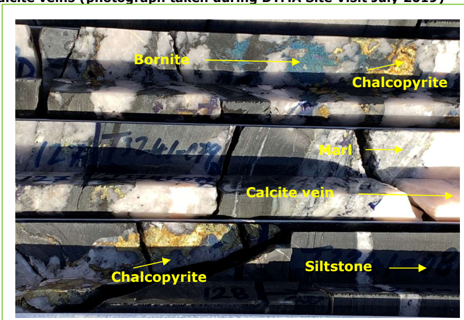
Figure 8 : Breccia-hosted, massive bornite and chalcopyrite within siltstone-marl host rock, which is cross-cut by calcite veins (photograph taken during DTMA Site Visit July 2019)
