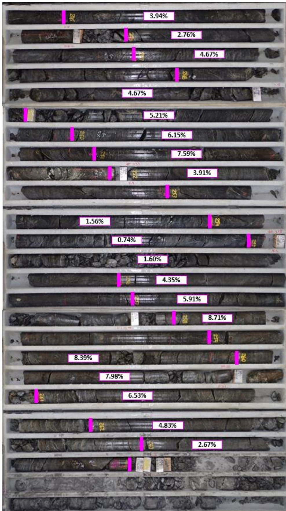
Photo 1 - U6966 DRILL CORE BETWEEN 245m and 265m SHOWING TIN ASSAY RESULTS
