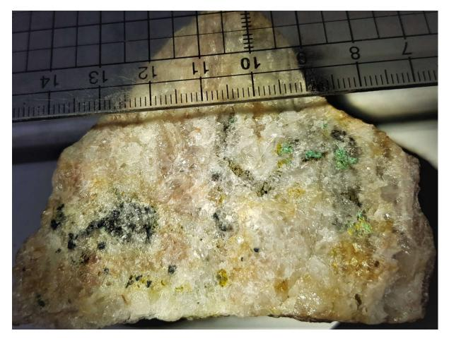
**Picture 5:** Mineralised quartz from the Thumbo epithermal vein at rock chip sample site SO33. This sample returned 551ppm Cu (although much of the copper was lost during sampling), over 2,000ppm Pb, 0.9g/t Ag and 84ppb Au.
