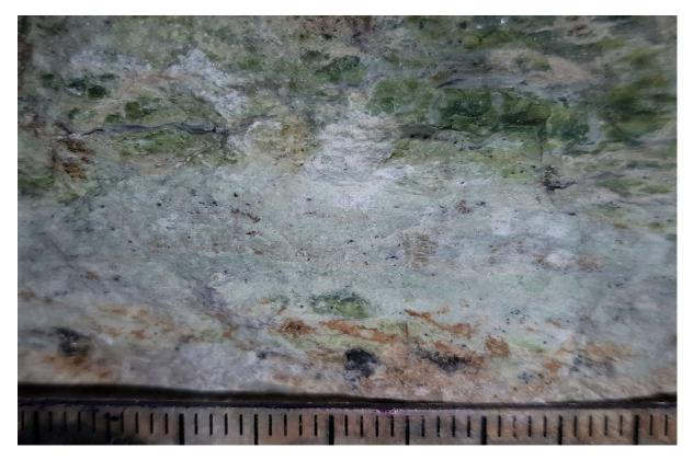
Picture 6: Calcrete from MG1 Apron, Sample 8 (Scale in mm).
