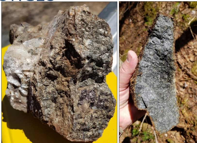
Figure 9: Quartz veining in Nipissing Diabase (left) and Nipissing Diabase hosting sulphide mineralisation (right)
