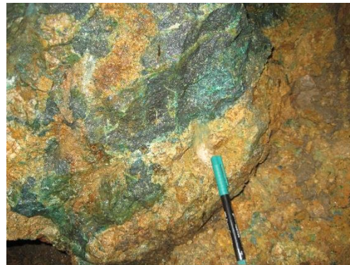
Sample 26625—27.2% Cu, 0.27%Co, 35.3g/t Ag, 0.32% Sb, 0.24% Ni
