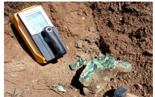
Sample 26584—37.5% Cu, 0.27% Co, 193g/t Ag and 0.14% Ni
