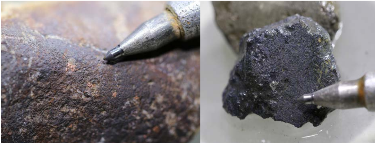
Figure 3: Native copper in MWAC0109 (left); chalcocite from MWAC0112 (right)
