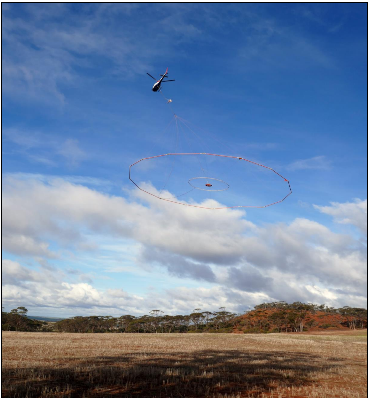
Fig. 2 Airborne geophysical survey - Wongan Hills (June 2018)
