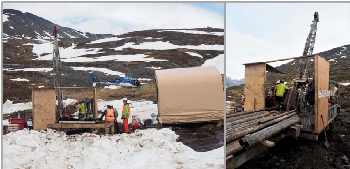
Figure 6 Helicopter portable drill rig in action at Zackly, July 2018
