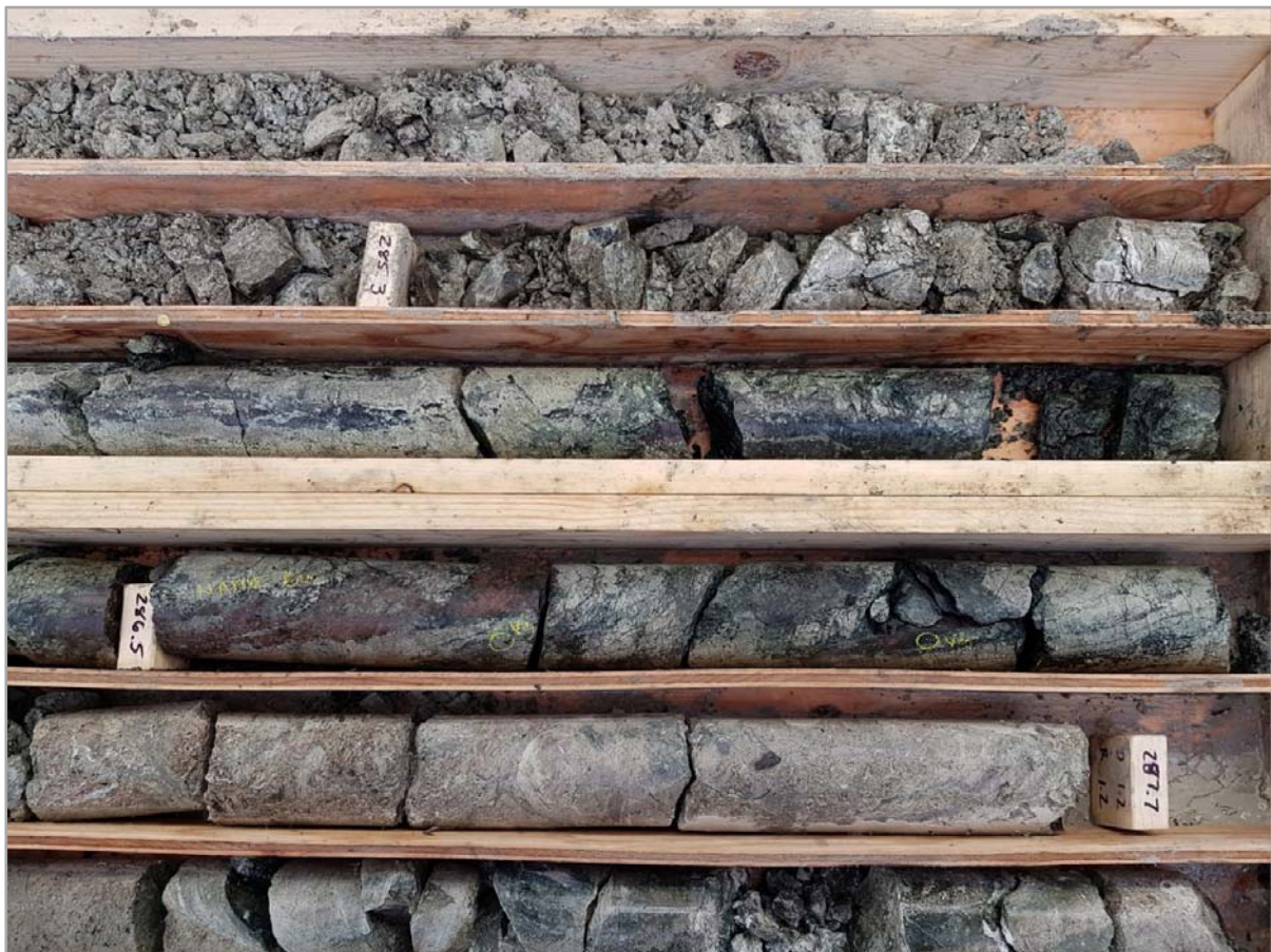
Figure 1. Visible copper, copper sulphides and native gold in hole ZX-18022, 284.0m to 288.5m down-hole depth. Visible gold grains circled
