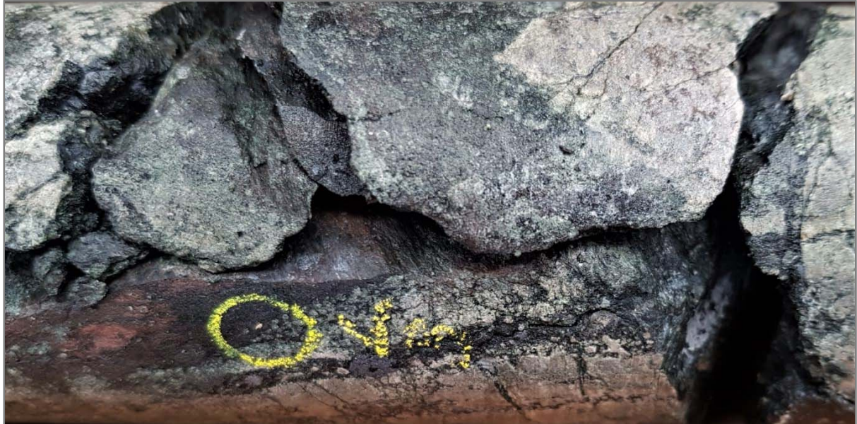
Figure 2 Visible gold grain associated with high-tenor copper sulphides and native copper in ZX-18018 at 286.9m down-hole depth.
