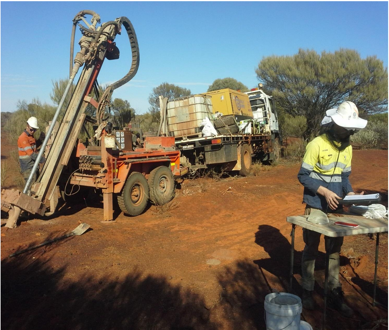
Figure 2: AC drilling on the Primrose Project, WA.
