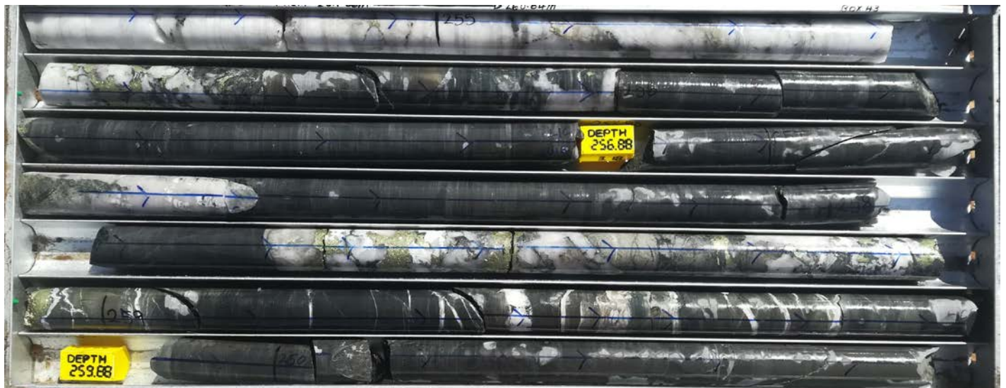
Figure 3: MO-A4-003D drill core from 254.6-260.6m depth showing chalcopyrite in quartz/carbonate veins
