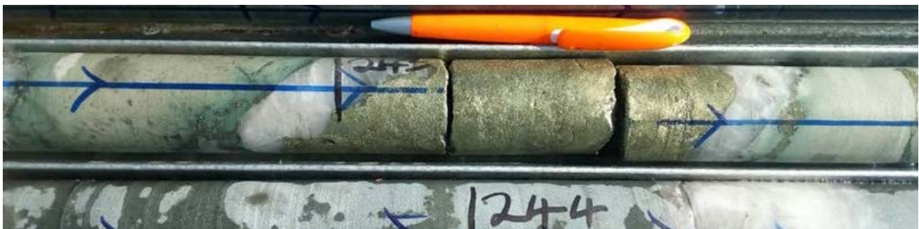
Figure 1: MO-A4-003D drill core at 243.1m depth showing massive chalcopyrite in quartz/carbonate vein
