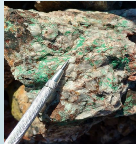
Secondary copper minerals and boxwork filled with mineralization
