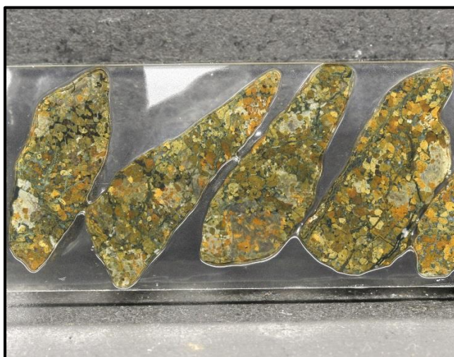
Photo 1 : Olivine-rich gabbronorite cumulate BOH petrology sample from RKAC255, 5cm width. (Photo taken prior to final thin section preparation).
