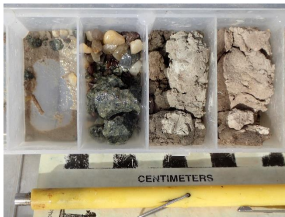
Figure 4 (A) Aircore hole MYAC153 (2010) eoh sample showing altered monzodiorite and pebble contamination. Sample assayed 0.22% Cu. (B) Drilling rig onsite this year.
