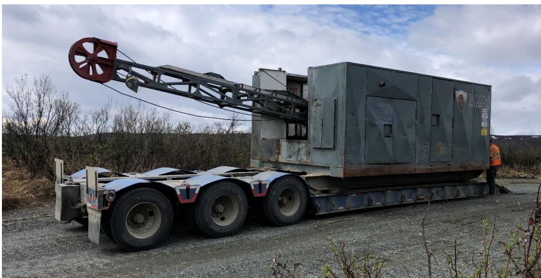
Figure 3 Skid mounted rig being prepared for final mobilisation to drill site
