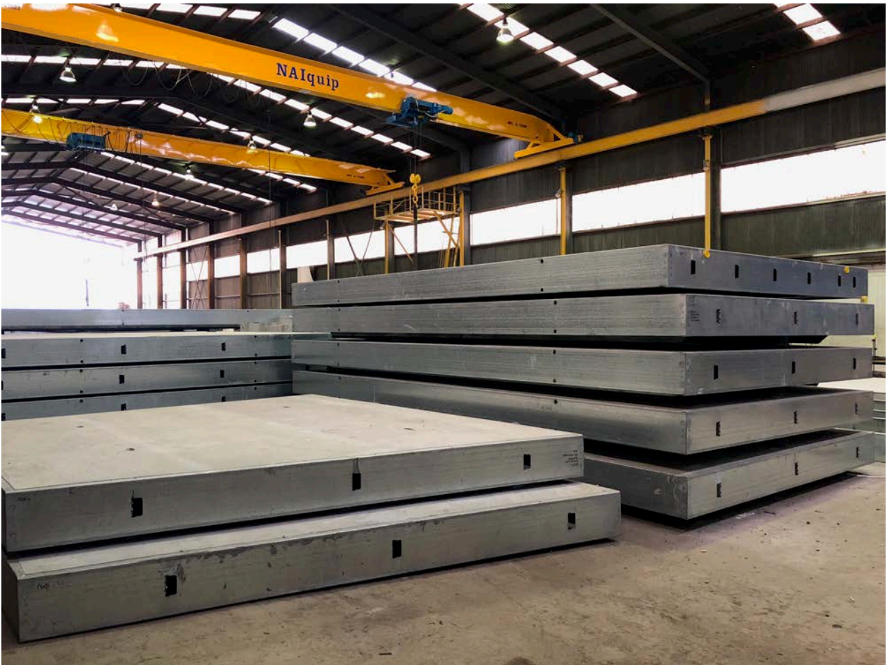
Stockpiled lightweight slab panels
