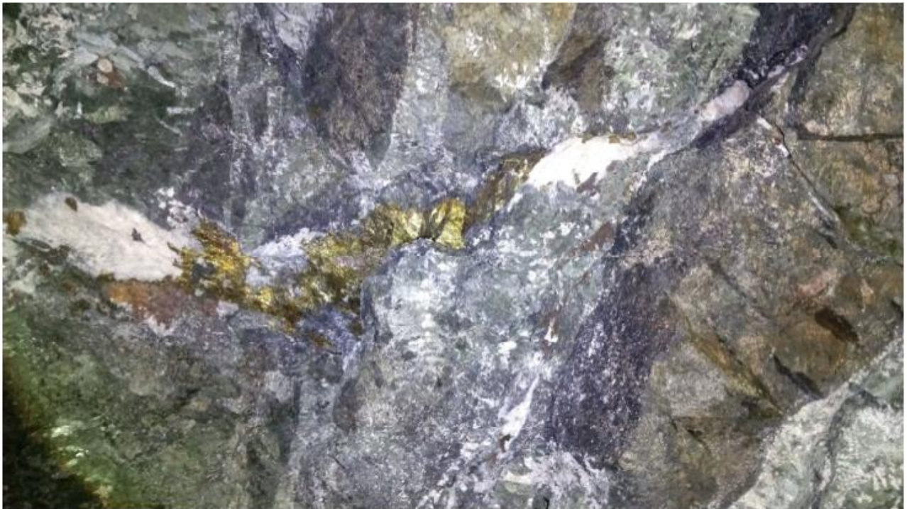
Figure 15 – Main vein, lowest level Mina Verde mine. Massive magnetite and chalcopyrite with calcite and actinolite. Note banding and filling of earlier voids with minerals (Source: Titan Field Trip, 2017)
