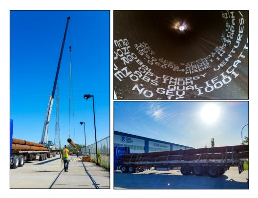
**Pictures Above:** The 28 lengths of 18m API Spec X80M pipe arriving at the C-FER Technology Testing Facility (<u>www.cfertech.com</u>). For testing purposes, 20" diameter pipe is being used as it will reduce the number of end fittings and overall cost. C-FER's facilities include a world-class laboratory in which full scale equipment qualification testing can be performed at high pressure, temperature and load conditions.
