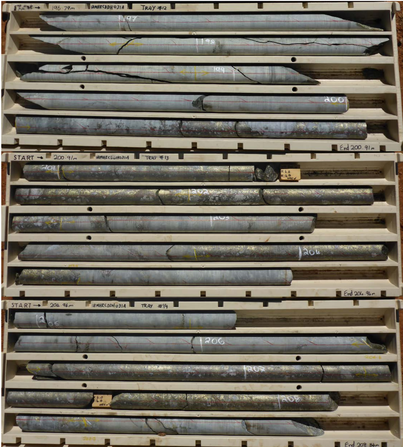
Figure 2 – Drill core from 18MHRCDH031A, showing the sulphide mineralisation from 196.8m to 209m depth. Yellow shiny core is chalcopyrite, while darker intervals are sulphide-dominated.
