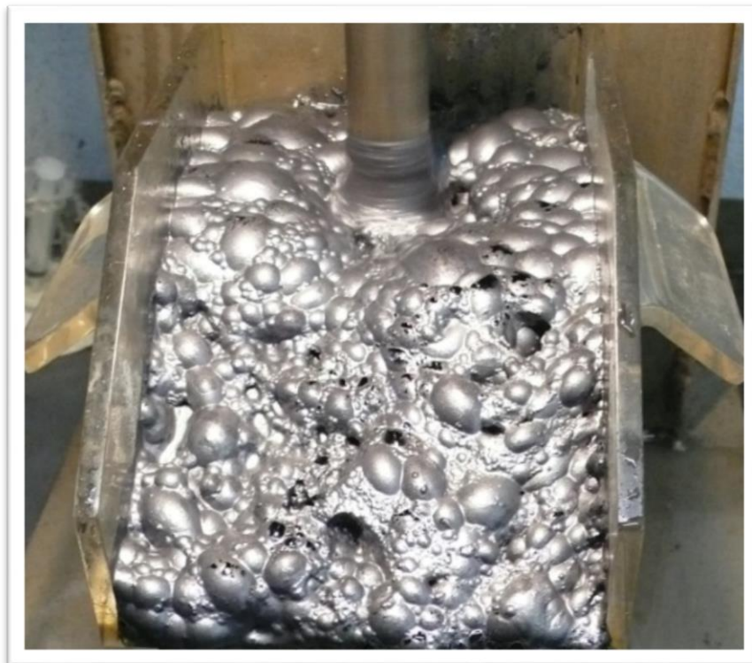
Figure 2: High-grade lead-silver concentrate from test-work on Abra samples.
