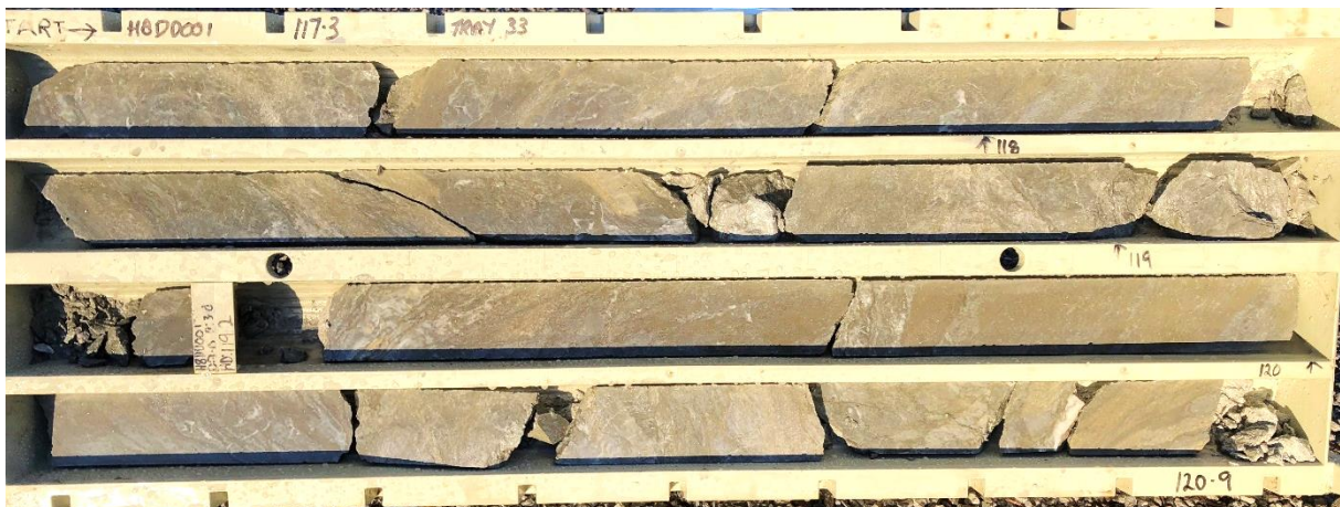
Figure 3: H8DD001 mineralisation (half-HQ core, 117.3 to 120.9m downhole).
