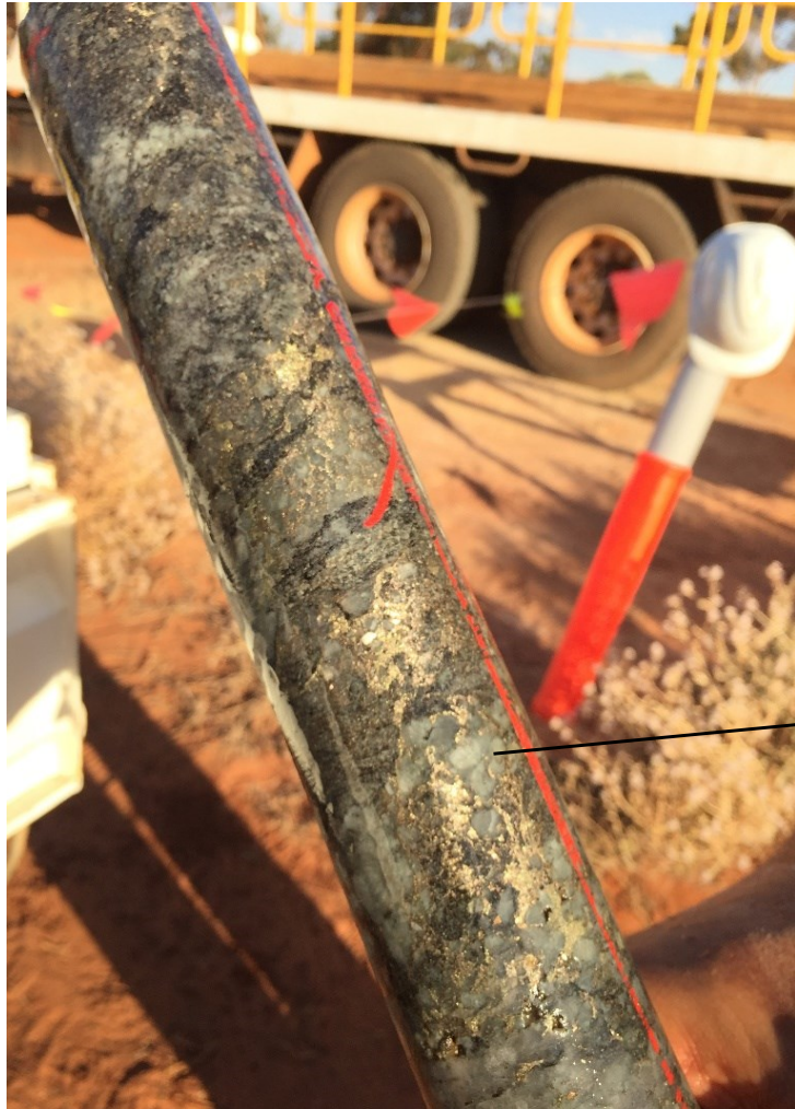
Pyrrhotite & pyrite in altered gneiss: RDH04 153-157m 15.20g/t
