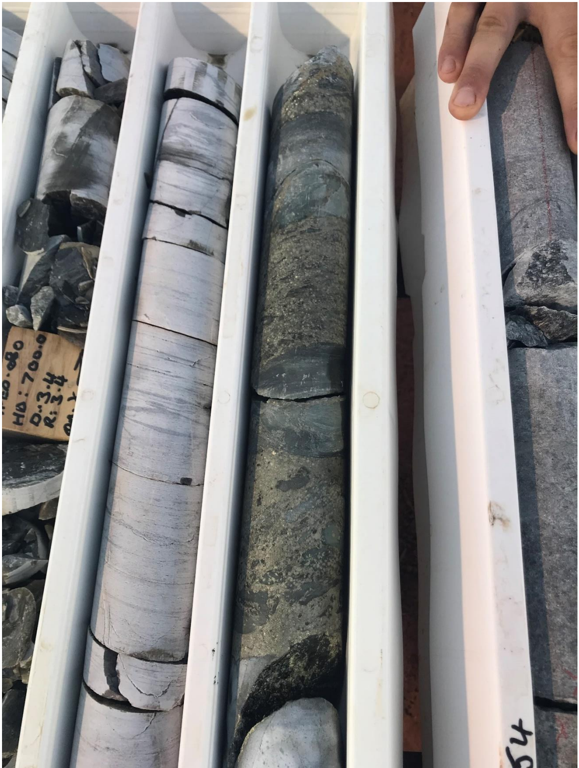
Photo of Musket massive sulphide grading 8.1% Ni from MFED080
