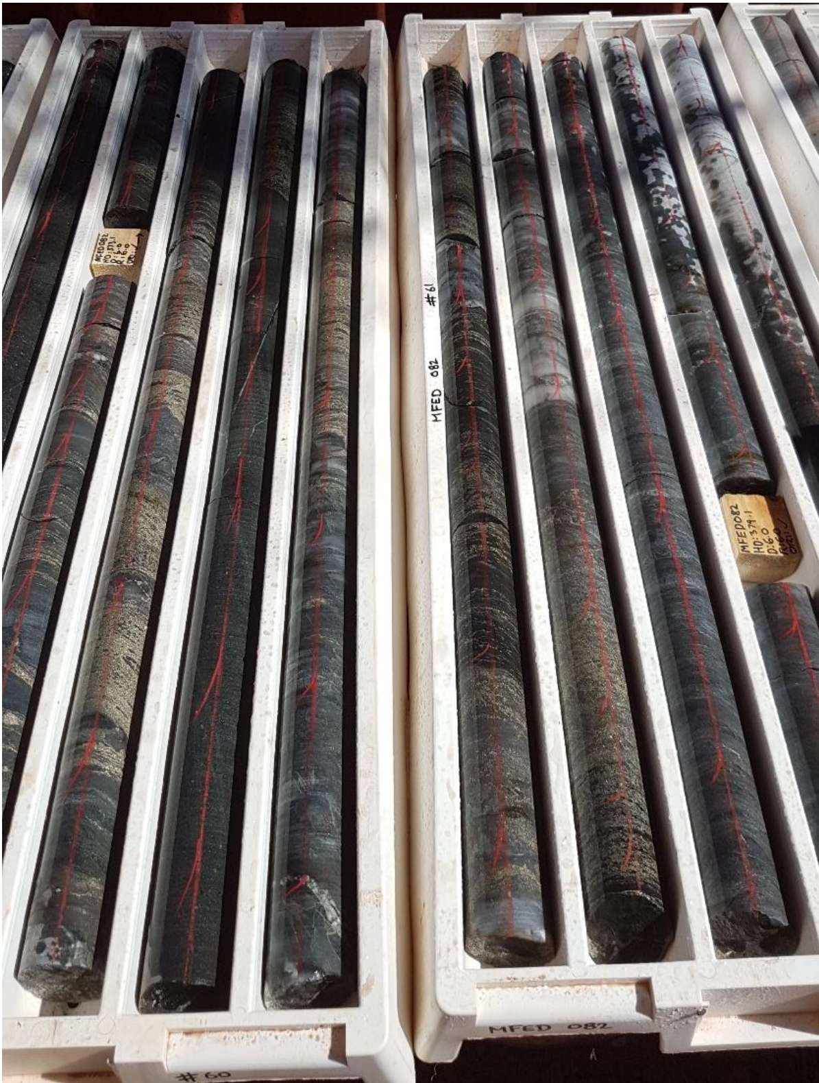
Photo of Corktree mineralization, pyrite-pyrrhotite-magnetite from MFED082
