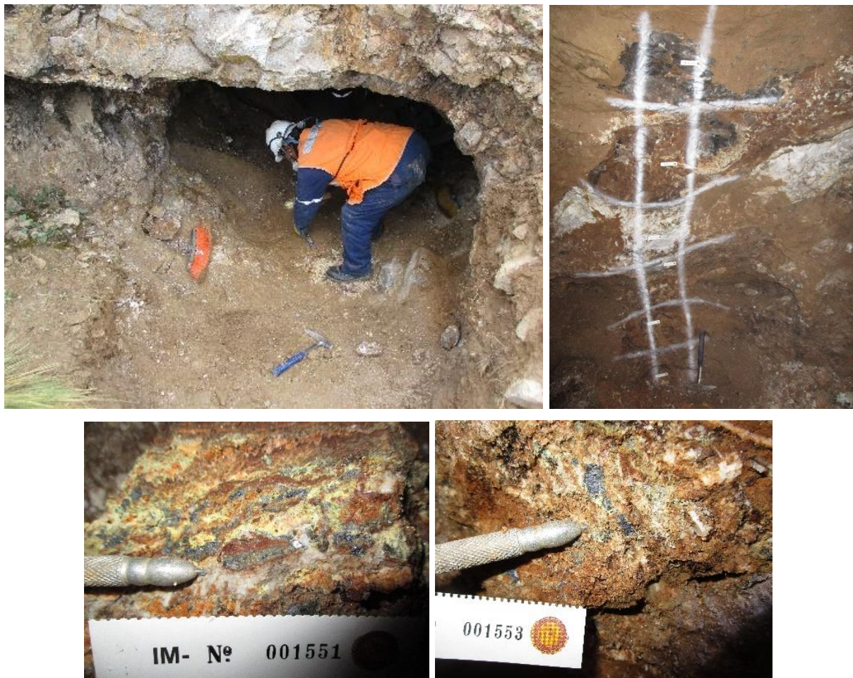
Selection of photos taken during the sampling program subject of this announcement. CLOCKWISE: Opening the adit to gain access to the interior of the underground mine; A typical line of samples that constitutes a “channel” – a continuous line of samples to obtain a continuous measure of the mineralisation; photo of IM-001551 with visible galena, sphalerite and smithsonite; photo of IM-001553 with visible galena, sphalerite and smithsonite.
