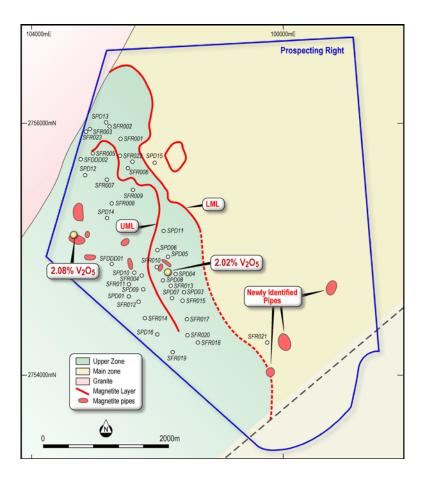
*Figure 5.* Plan showing location of surface samples and magnetite pipes at the SPD Vanadium Project along with historical drilling and geology.
