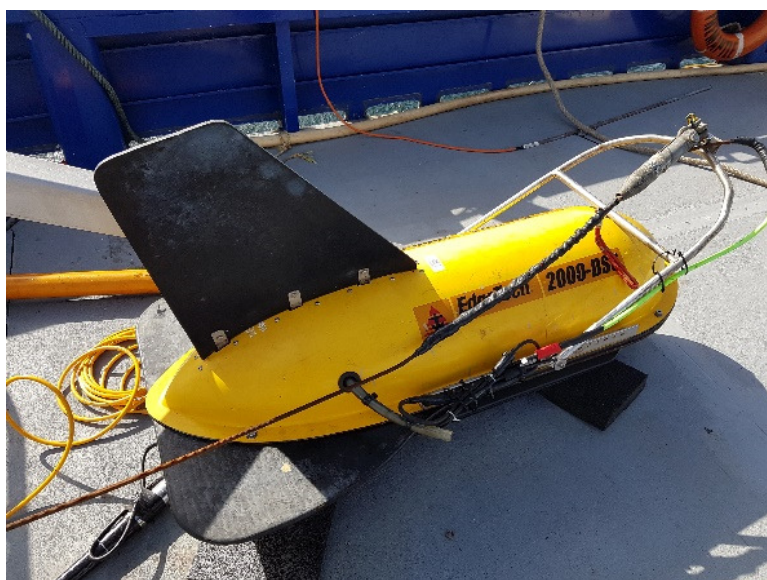
Chirp and Side Scan Sonar System (left) and Business Class vessel surveying in Torbay, Albany (right)
