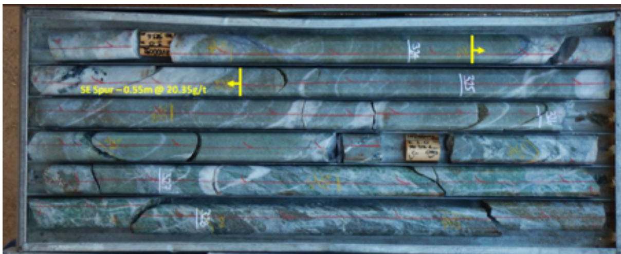
Figure 5: South-East Spur intersection in 18VIDD092 with interval and grade shown in yellow.
