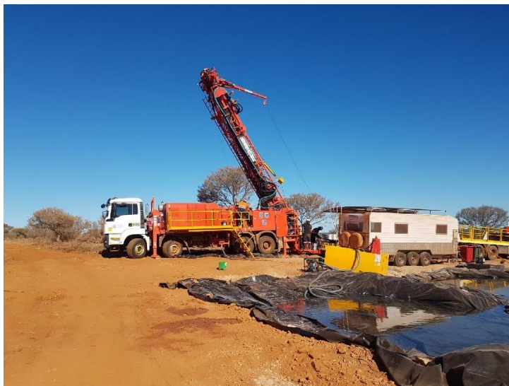
Figure 1 Diamond Drilling Underway at Saturn Metals' Apollo Hill Prospect – 29 May 2018.
