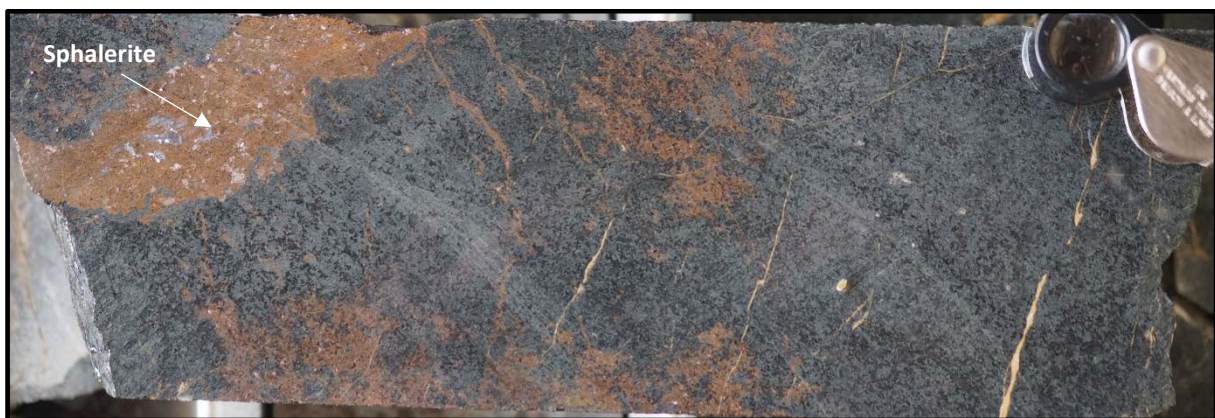
Figure 5. Sphalerite and galena in extensional veinlets (JBDD002: 96.27-96.46m).
