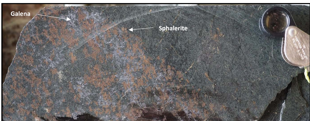
Figure 6. HQ half core (JBDD002: 95.58-95.8m), chloritic rock with stringers of sphalerite (brown-red) and galena (grey).
