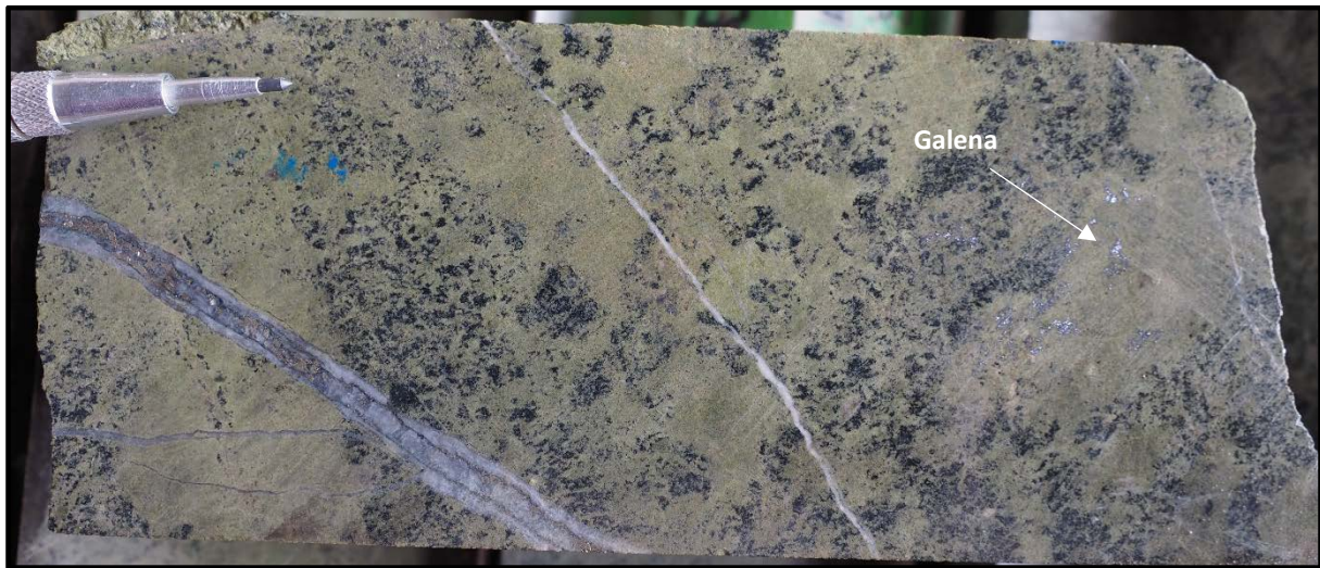
Figure 4. Galena bearing ore horizon (JBDD003: 53.4-53.55m): Disseminated galena to right side of image, with cross cutting pyrite vein on left.
