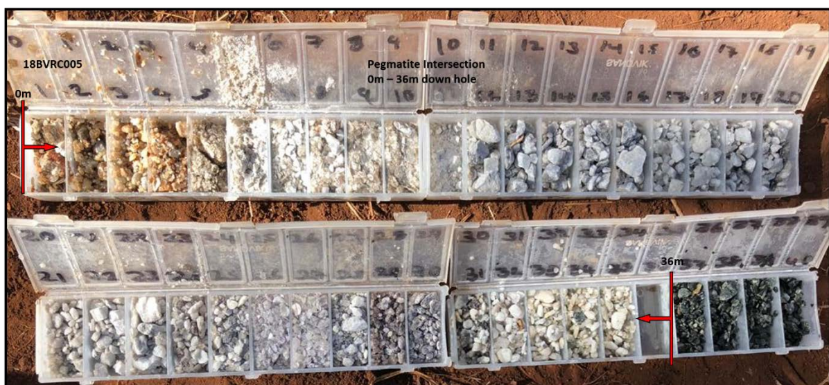
Figure 1: Pegmatite intersection in from hole 18BVC005. The pegmatite extends from surface to a depth of 36m and contains a high content of lithium minerals spodumene and lepidolite. Note that the hole drilled sub-parallel, or down-dip, of a pegmatite dyke
