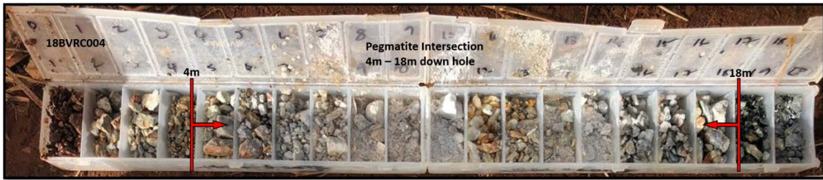
Figure 2: Pegmatite intersection in from hole 18BVRC004. The pegmatite extends from 4m to a depth of 18m and contains a high content of lithium minerals spodumene and lepidolite. The hole was drilled perpendicular to the strike of the pegmatite dyke.
