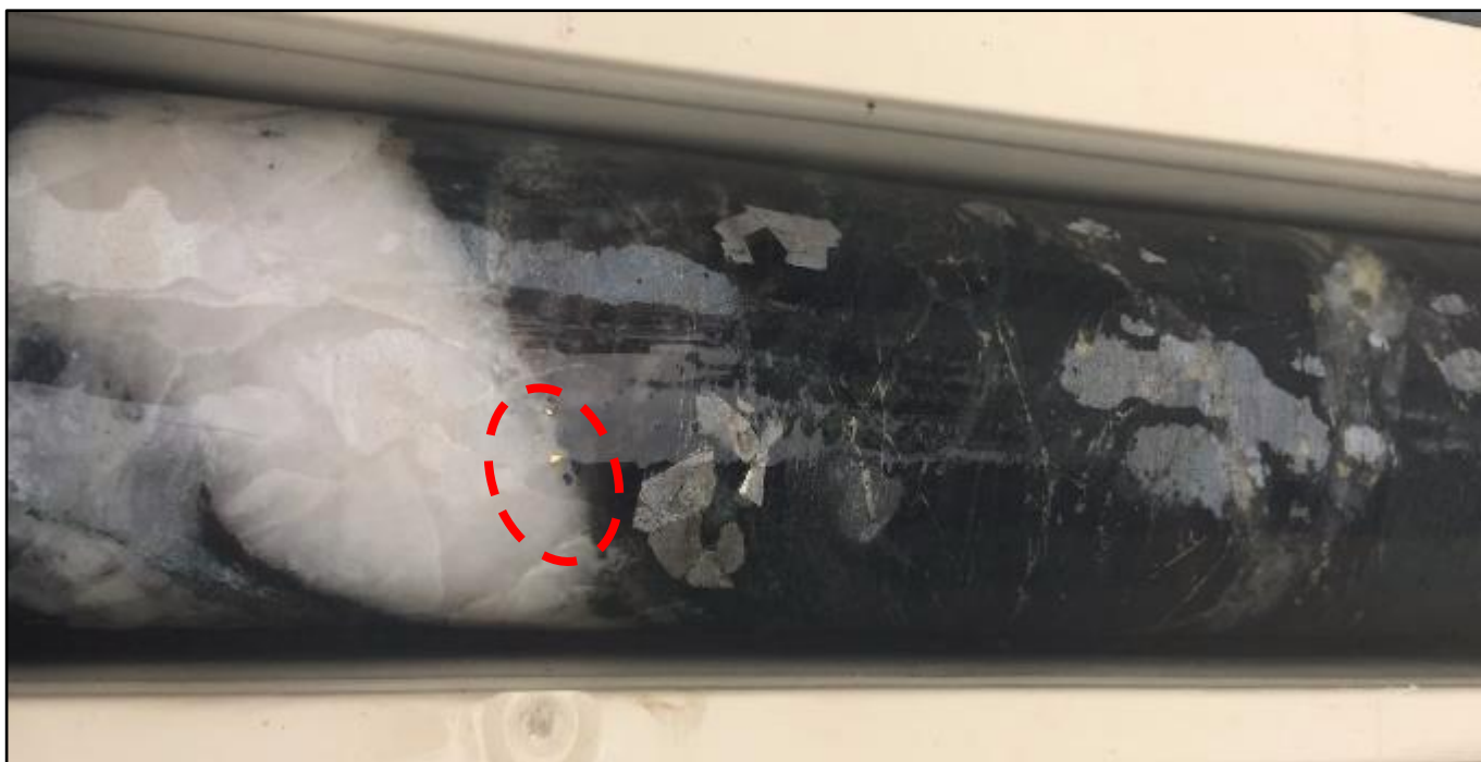
Figure 6: RD013 drill hole with visible gold (inside red circle) and coarse-grained arsenopyrite intersected.
