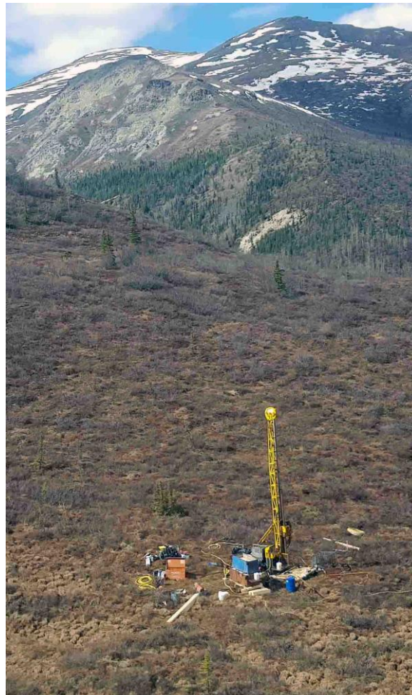
Figure 2: Diamond drill rig set-up at West Tundra Flats.
