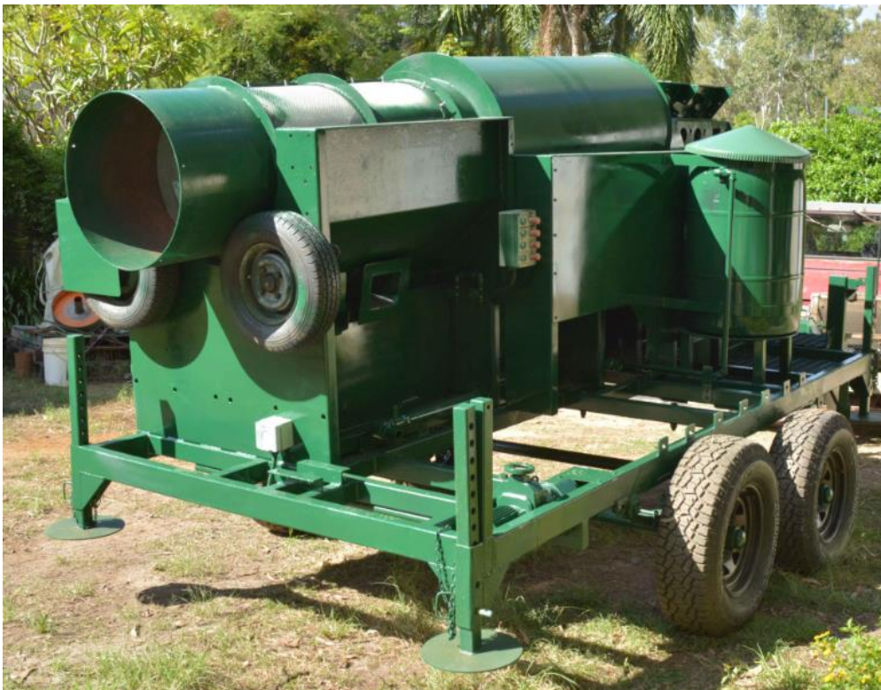
Figure 9: View of trommel and wet scrubber of mobile gravity gold bulk sampling plant
