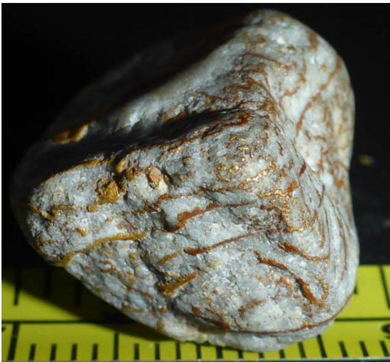
Figure 4: Wire gold clearly shed from a high grade gold source. Scale in both inches and centimetres
