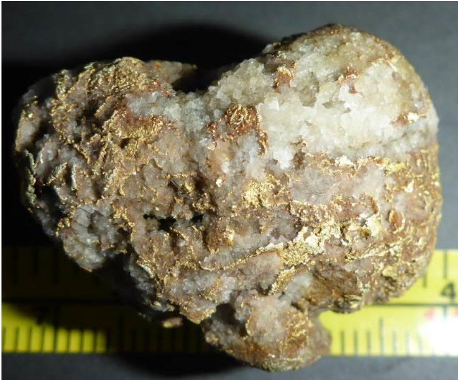
Figure 1: Bonanza-type gold indicative of boiling zones of epithermal gold deposits. Note quartz consists of interlocking prismatic ‘sugar grain-sized’ crystals that grew in an open-spaced epithermal environment. Such delicate specimens are close to source and would quickly disintegrate when water transported with large boulders. Scale in both inches and centimetres.
