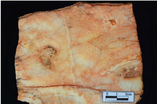
Photo 7: KRS203141. 1.56 g/t Au, <2 g/t Ag Limonitic to haematitic recrystallised chalcedonic quartz with a cockade band rimmed rhyolitic wall-rock fragment. North Beopseongpo Vein Segment.
