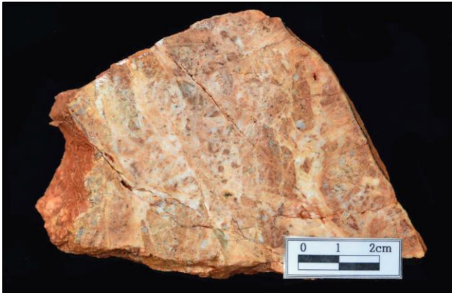
Photo 3: KRS203143. 0.38 g/t Au, <1 g/t Ag. Hydraulic vein breccia comprised of angular rhyolitic wall-rock fragments set in a white mesocrystalline quartz flood matrix. North Beopseongpo Vein Segment.
