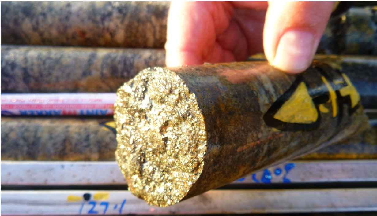
Figure 3: An example of the strongly pyritic (potentially cobaltiferous) bands in albitic gneiss in DD95STV3.
