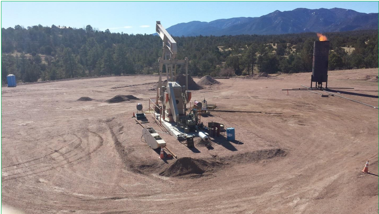
Figure 1: Pathfinder horizontal well flow testing and flare from the Niobrara Formation
