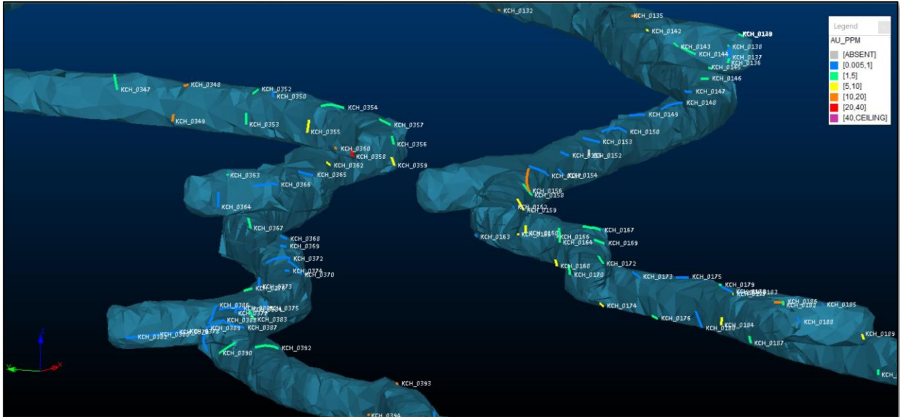
Figure 4: Isometric image showing 3D laser modelling of old workings with channel samples highlighted along the 245 Level Drive 1 & 2 West.
